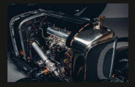
Every single component was laser scanned and new ones were then hand crafted. Bearing in mind this includes all the interior workings of the engine and supercharger, plus the dials, trim and numerous fixings, it's easy to see why construction of this new Bentley Blower has taken so long.
